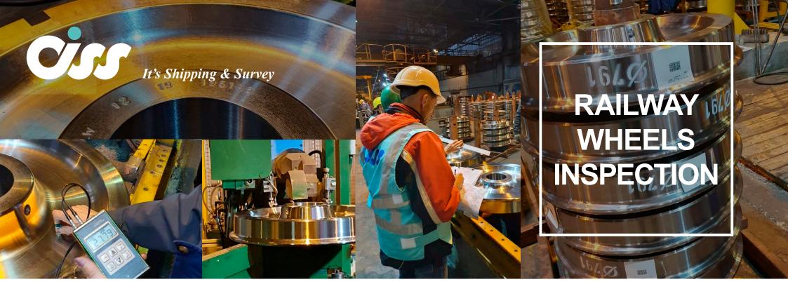
Wheels are cast or forged and are heat-treated to have a specific hardness.
